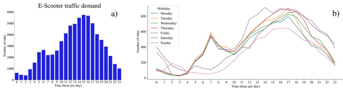
Figure 2 – Hourly e-scooter traffic demand in Ingolstadt with a) over all weekdays accumulated and b) filtered for each weekday.
