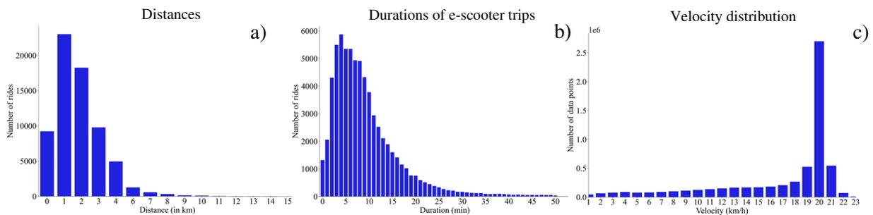
Figure 1 – Shared e-scooter ride histograms with a) driven distances, b) trip durations and c) velocities of the datapoints as described above in Methodology.
